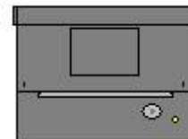
The panel mount printer uses thermal heat transfer technology. The single button is for form-feed. To tear paper, pull towards the front of the instrument along the serrated cutting edge.
